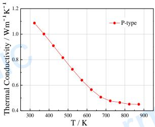
Thermal conductivity of the SnSe-based ingot
