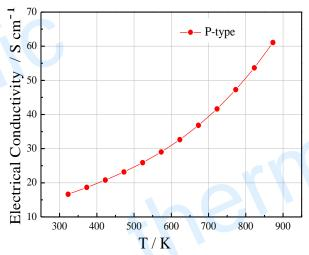
Electrical conductivity of the SnSe-based ingot
